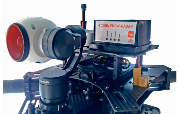
DK-sR-14MPe Monopulse Radar with Ethernet Interface mounted on an UAV
