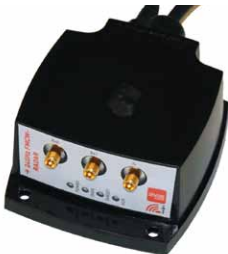
sR-1030 with RPC-2.92 connectors for external antennas (one Tx, two Rx)
